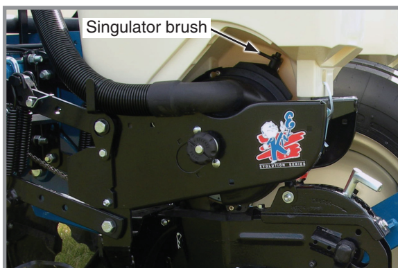
Singulator brush adjustment location
