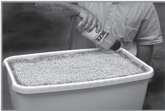
Adding graphite to conventional hopper
