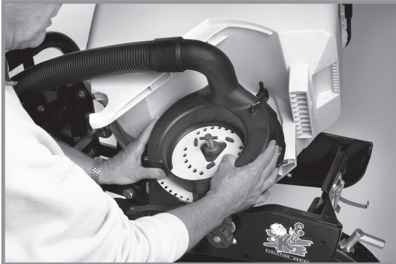
Remove vacuum cover and seed disc
